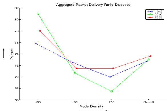
Figure 14: Packet delivery aggregate statistics for different node densities
