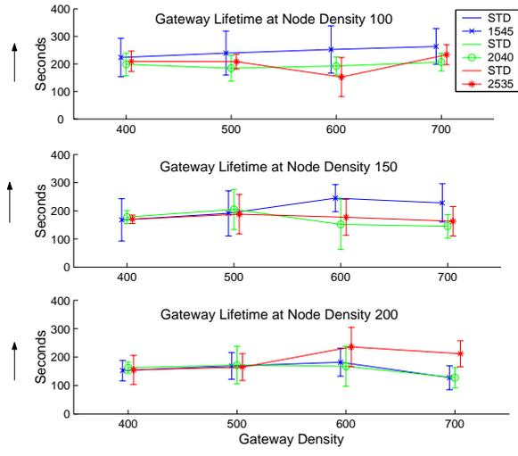
Figure 5: Gateway lifetimes for different node and gateway densities
