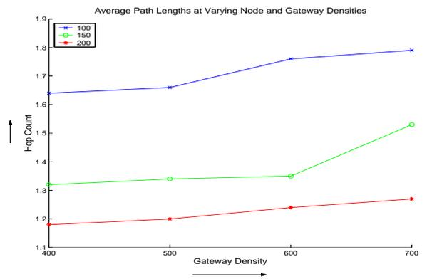
Figure 15: Average path lengths for varying gateway densities
