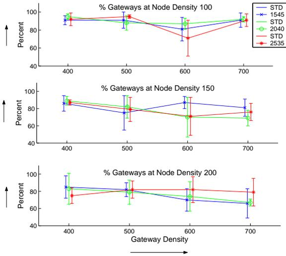
Figure 9: Percentage of time gateways were available for different node and gateway densities
