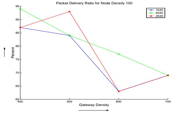
Figure 11: Packet delivery ratio statistics for a node density of 100
