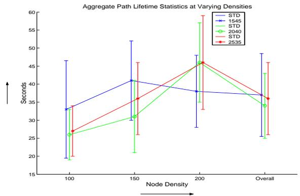
Figure 4: Path lifetime aggregate statistics for different node densities
