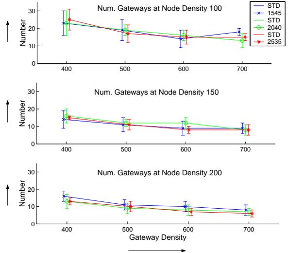
Figure 7: Number of gateways for different node and gateway densities
