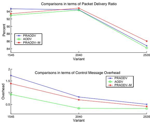
**Figure 19: Comparisons in terms of packet delivery ratio and overhead**
