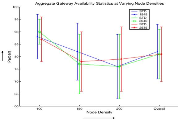
Figure 10: Gateway availability aggregate statistics for different node densities
