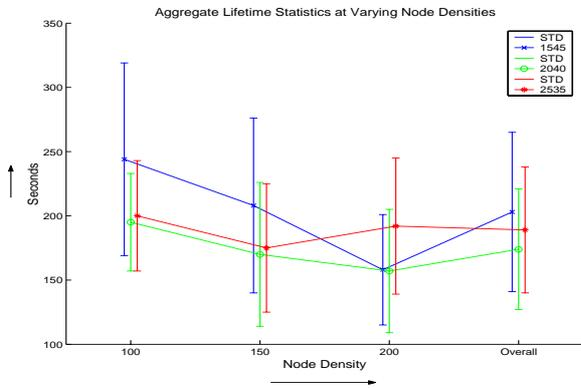
Figure 6: Gateway lifetimes aggregate statistics for different node densities
